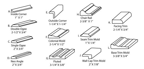
Solid cast moldings should be fastened in place with adhesive.
